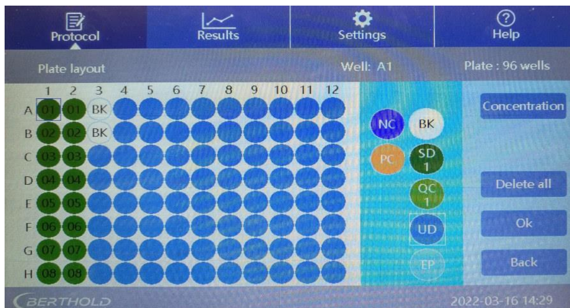
Figure 2. Plate layout programmed in the Apollo software. Wells in green are the standards (Standard 1 to Standard 8), wells in white are the blanks, and the rest of the plate is left for samples. The unknown sample was pipetted in duplicate in wells C3 and D3.
