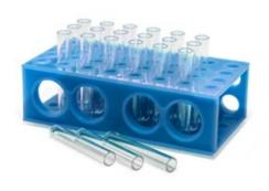
We offer sample tubes for luminescence detection in different heights/volumes, which are suitable for measurements in tube luminometers. The tubes are made of polystyrene, have a diameter of 12 mm and fit all our tube luminometers.
